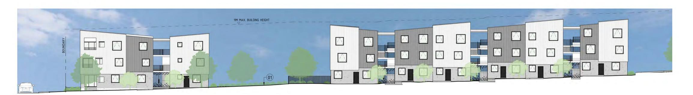
LEGEND PRECAST CONCRETE STRUCTURE VERTICAL ALUMINIUM CLADDING VERTICAL ALUMINIUM CLADDING DOUBLE GLAZING PROFILED METAL ROOFING LANDSCAPING
