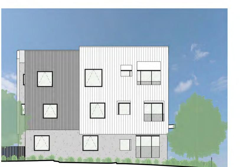
LEGEND PRECAST CONCRETE STRUCTURE VERTICAL ALUMINIUM CLADDING VERTICAL ALUMINIUM CLADDING DOUBLE GLAZING PROFILED METAL ROOFING LANDSCAPING
